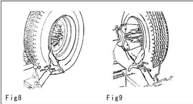
4. Turn the tire and meanwhile move the circular bead breaker disk (12) forward.
